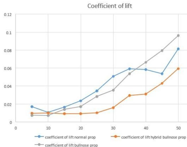
**Fig. 14 Coefficient of lift VS air speed**
