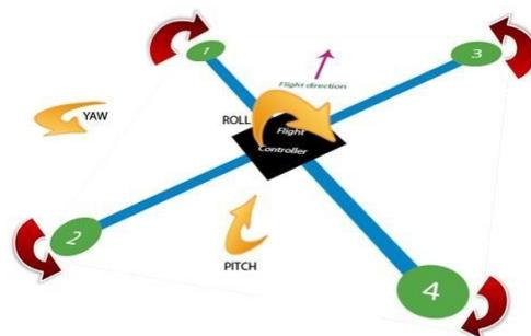
Fig. 1 Movement of a quadcopter
