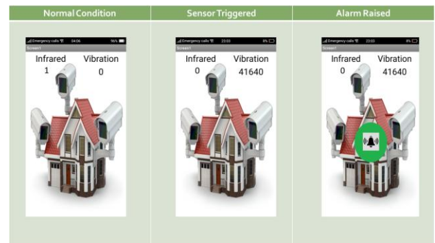
Fig. 6 Mobile application show the data receive from ThingSpeak and alert the user
