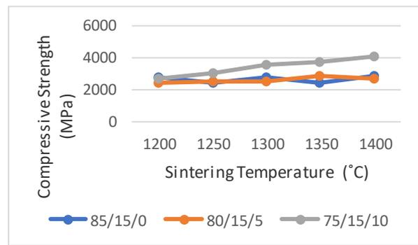
**Fig. 3 The effect of various compositions and sintering temperatures on the compressive strength of zirconia for 1.5h holding time**
