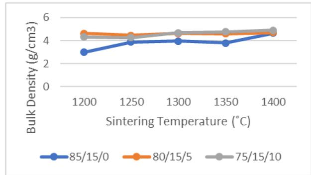
**Fig. 1 The effect of various compositions and sintering temperatures on the bulk density of zirconia for 1.5h holding time**
