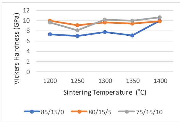
**Fig. 2 The effect of various compositions and sintering temperatures on the Vickers hardness of zirconia for 1.5h holding time**
