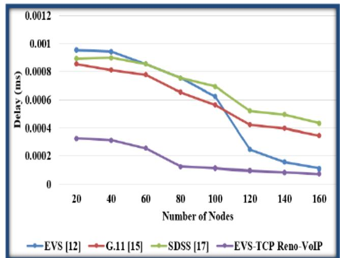
**Fig. 7 Comparative analysis of delay performance for an existing and proposed method**
