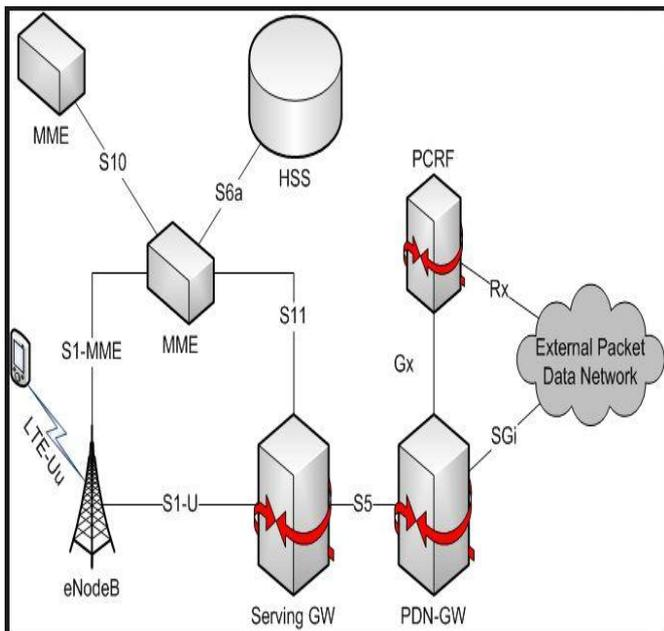
Fig. 3 The architecture of the packet data network
