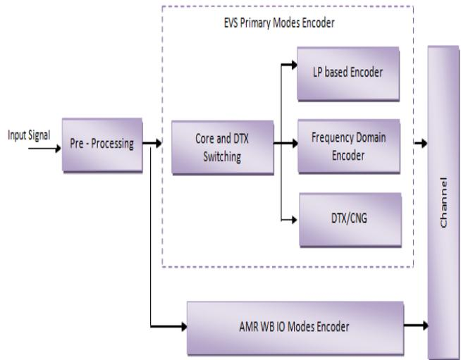
Fig. 4 Block diagram of the EVS encoder process
