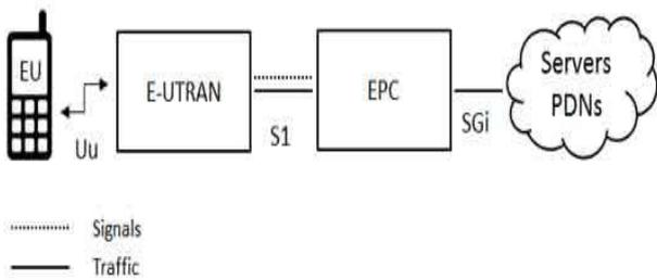
Fig. 1 The architecture of the LTE-A
