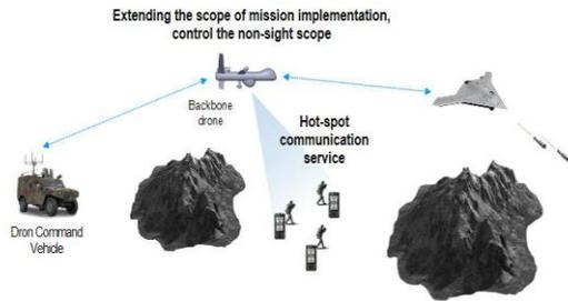
**Fig. 7 A Concept of the network configuration using backbone drones**
