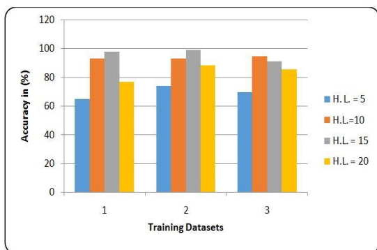
Fig. 6. Accuracy of ANN numeral classifier during different training session with varying number of hidden layers
