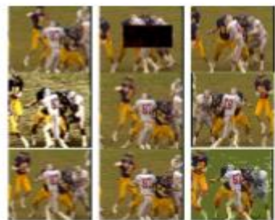
Fig.6. (a) Unsharp filtering, (b) Cropping to one-eighth portion of frame of video (c) Smoothing (d) Histogram Equalization (e) Rotation by 5° (f) Sharpening (g) Blurring due to camera movement (h)Circular Blur(g)H.264 Compression
