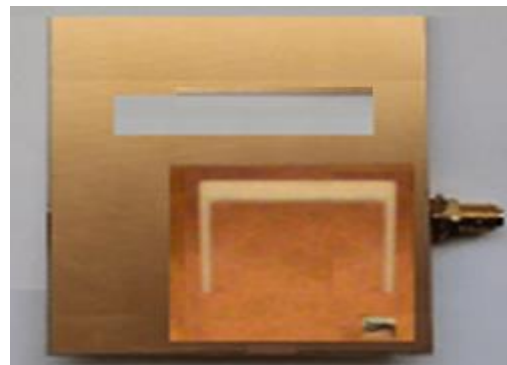
Figure 2. The proposed PIFA prototype
