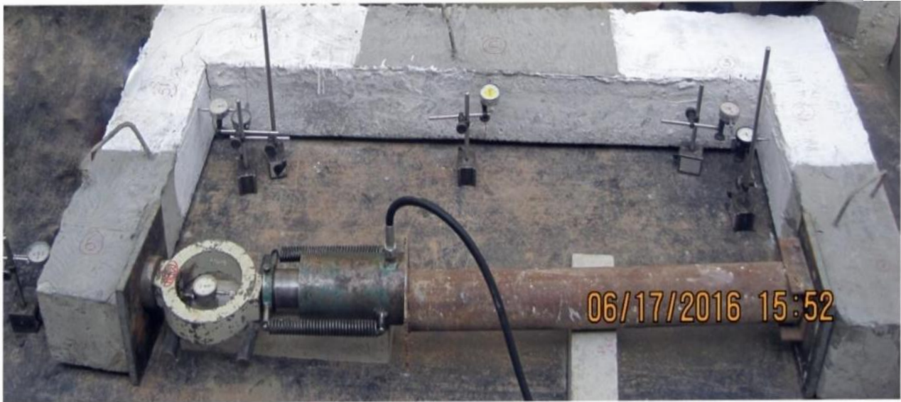
Figure 3 Testing of SFRC Joint Model
