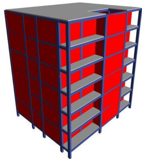
Fig 3b: G+5 RC Structure with Infill
