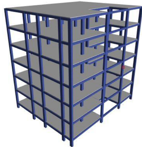
Fig 3a: G+5 RC Structure without Infill
