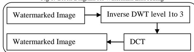
Fig 2. Block Diagram for Watermark Extraction
