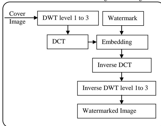
Fig 1. Block Diagram for Watermark Embedding
