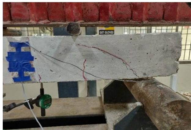
Fig. 3 Crack Pattern (Front)
