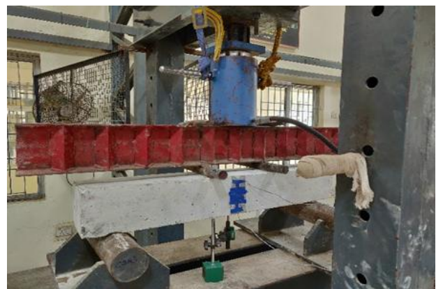
Fig. 2 Flexure specimen Test setup
