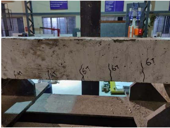
Fig. 4 Crack Pattern (Back)
