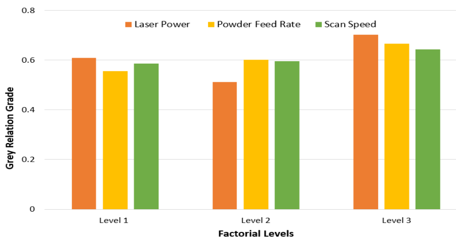
Figure3: Response chart for Grey relation grade of hardness, wear and corrosion rate
