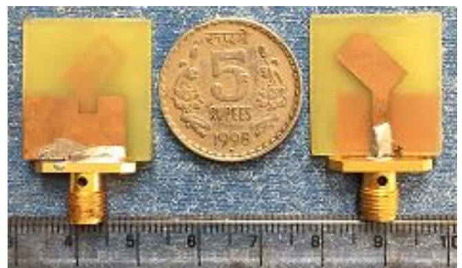
Fig. 2. Rear and front view of printed antenna
