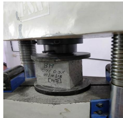
Fig. 3 Compression test setup of cube
