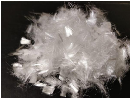
Fig. 2 PPF of 6mm length and 0.01 mm diameter
