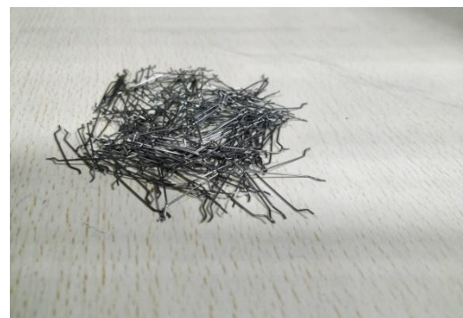
Fig. 1 HESF of 30mm length and 0.5mm diameter
