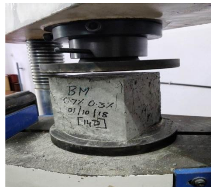
Fig.4 Failure mode of Cube specimen
