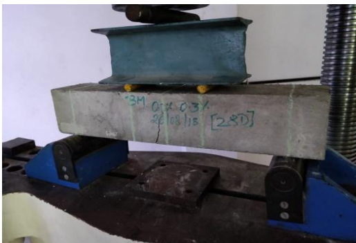
Fig.8 Flexural Test on Beam Specimen
