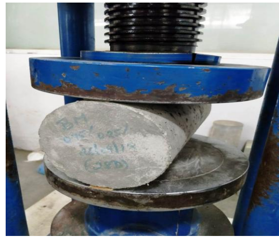
Fig.6 Testing of Cylinder Specimen
