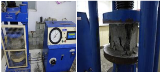
Fig. 5 Compression test (a) Testing of specimen in CTM (b) Failed specimens
