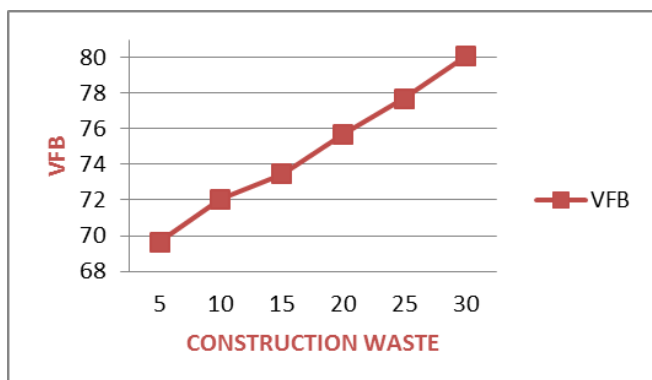
FIGURE 2: Effect of construction waste on voids on volume of mineral aggregates of bitumen mix
