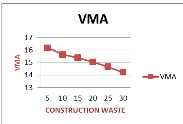
FIGURE 2: Effect of construction waste on voids on volume of mineral aggregates of bitumen mix
