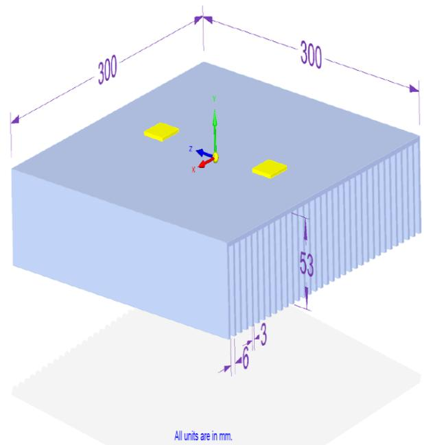
Figure 4: Design of the Heat Sink
