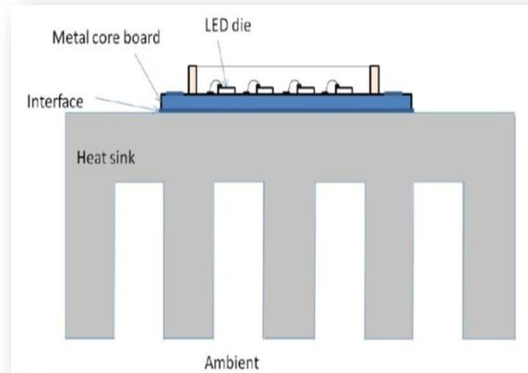
Figure 3: The basic structure of heat sink
