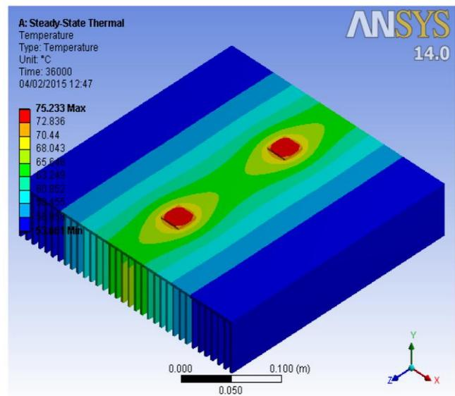
Figure 6: Heat Sink and Fins Thermal Analysis
