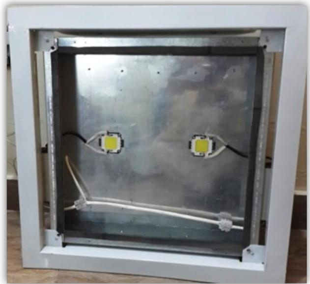
Figure 1 Canopy frame with COB LEDs
