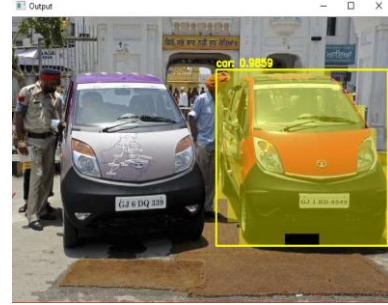
Fig 28. Blending the mask with colour.
