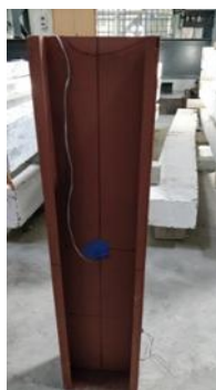
(a) Buckling of the specimen (BB200-S0-C20-3)
