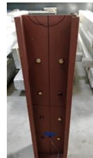
(b) Buckling of the specimen (GBB200-S25-C20- 4)
