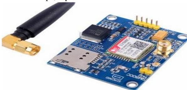
Figure.4. GSM Module
