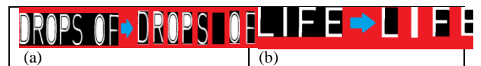
Fig. 5 Extraction of characters from words (a) Words segmentation for 1st section (b) Words segmentation for 2nd section.
