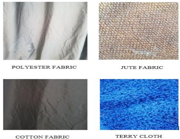
Figure 4. Various wick materials used in the still.
