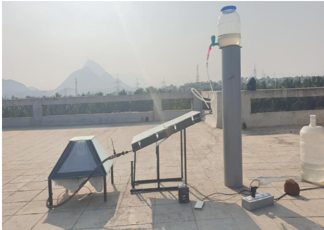
Figure 3. Pictorial View of Four Slope Solar still and parabolic reflector
