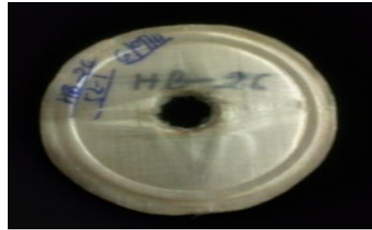
Fig. 6(a) Impacted specimen of HB-26 for 5L.
