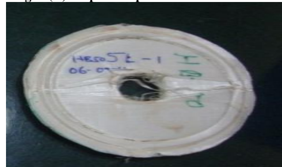
Fig. 6(d) Impacted specimen of HB-50 for 6L.
