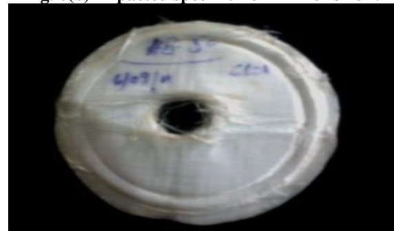
Fig. 6 (C) Impacted specimen of HB-50 for 5L.
