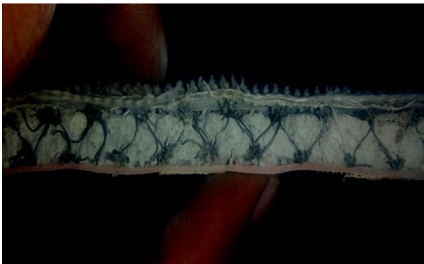
Figure 7: Side view of CC specimen showing bonding of fibres with the concrete.
