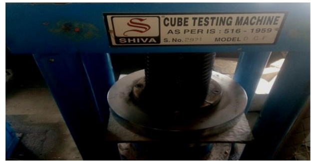
Figure 8: Universal testing Machine for Compressive strength of a material.
