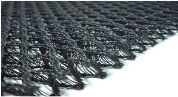
Figure 3: Showing the 3-dimensional Air mesh fabric Hydrophilic Sheet:
