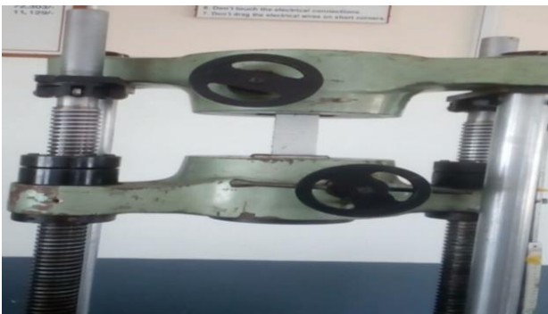
Figure 13: UTM for tensile strength of a specimen (CC)
