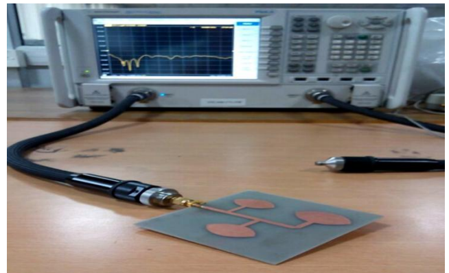
Fig 6 : Measurement of the S-Parameter
