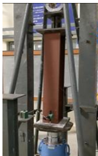
15 (a) Test setup of the specimen (BB200-S0-C20-3)
