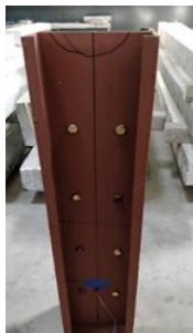
16(b) Buckling of the specimen (GBB200-S25-C20- 4)
