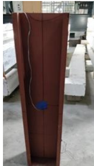
16(a) Buckling of the specimen (BB200-S0-C20-3)
