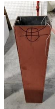
16(c) Buckling of the specimen (FF200-S0-C20- 3)
