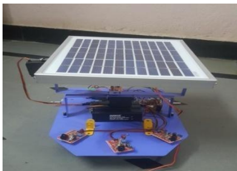
Fig: 6 Battery replaced with solar panel
