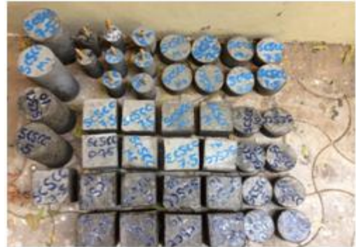
Fig. 2 Self-curing of SCC
