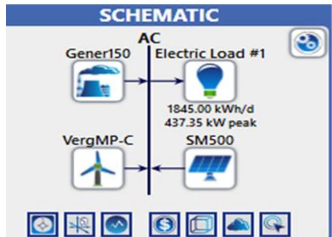
Figure 8: Model of the hybrid system in HOMER
