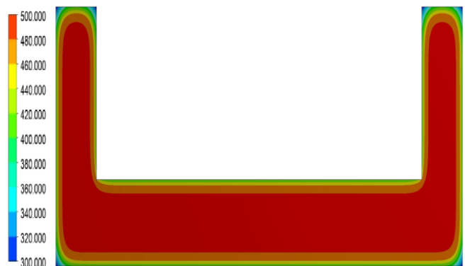
Fig. 3: Temperature field of semisolid cast part after quenching for 30 s
