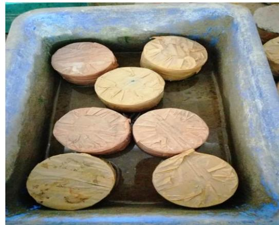
Fig 8. Sorptivity specimen
