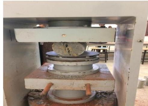
**Fig 3 split tensile strength**
