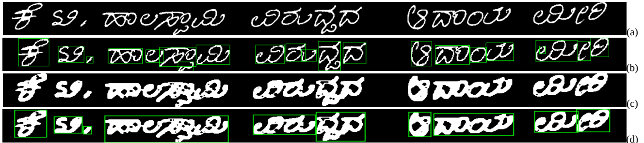
Figure 5: (a) 8 th segmented line using proposed binarization and segmentation technique. (b) Connected component technique on proposed system. (c) 8 th segmented line using Haar Wavelet Decomposition technique binarization and segmentation (Previous proposed technique). (d) Connected component technique on previous binarization technique.
