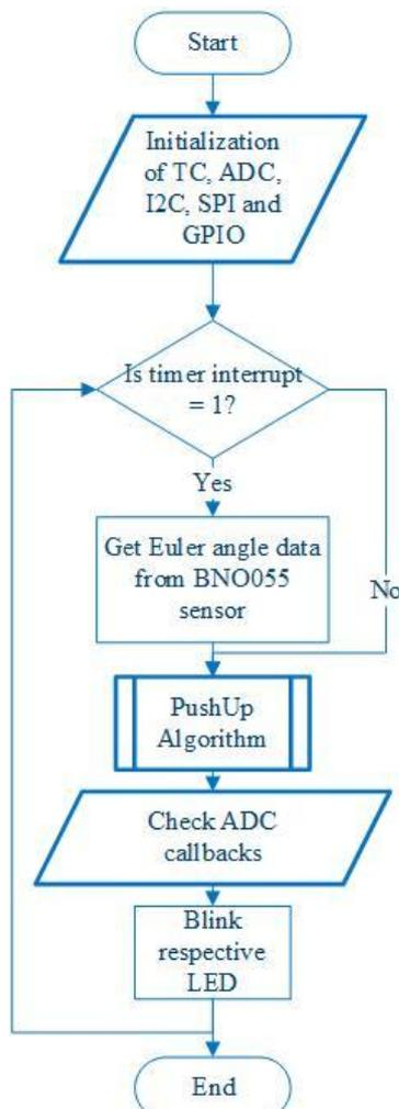
Fig. 3: Software control flow
