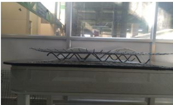
Figure 2- Shear connector welded with mesh
