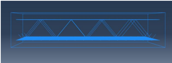
Figure 11- Schematic view of Foamed sandwich panel
