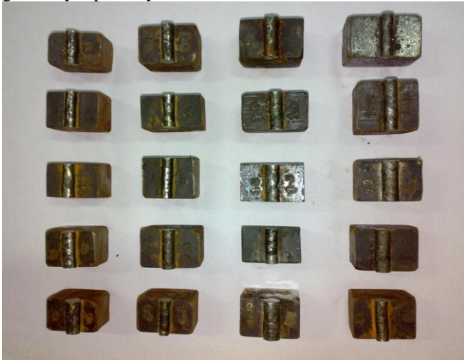
Figure 1: Photograph of cladded specimens
