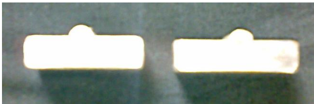
Figure 2: Typical cladding cross sections
