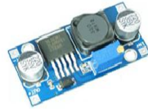
Fig. 7. DC to DC Converter: LM 2936
