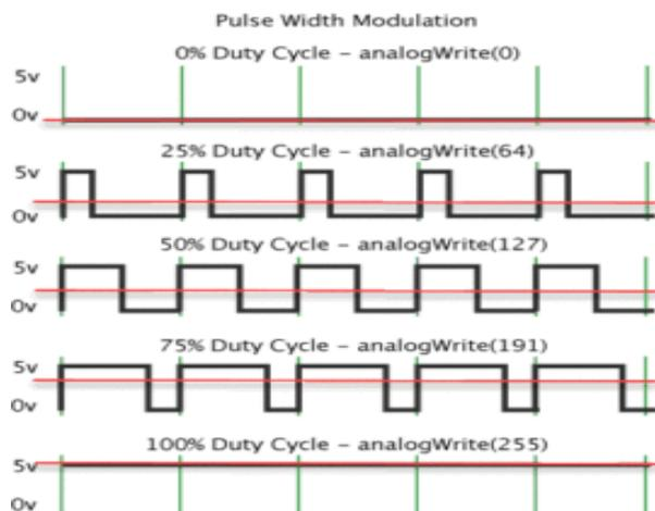
FIGURE 7: AN EXAMPLE OF A PWM SIGNAL SHOWN AT SEVERAL DUTY CYCLES AND A HIGH VOLTAGE LEVEL OF 5 VOLTS. THE RED LINE IS THE AVERAGE VOLTAGE THAT THE DRIVEN DEVICE (E.G., A MOTOR) IS EXPERIENCING.
