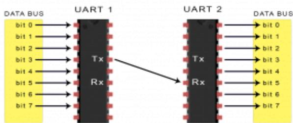
Fig 4 . PIN DIAGRAM OF UART
