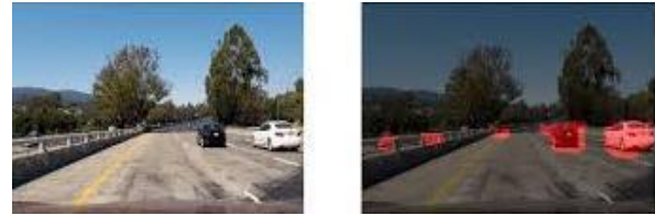
Figure 4: Car detection in an image
