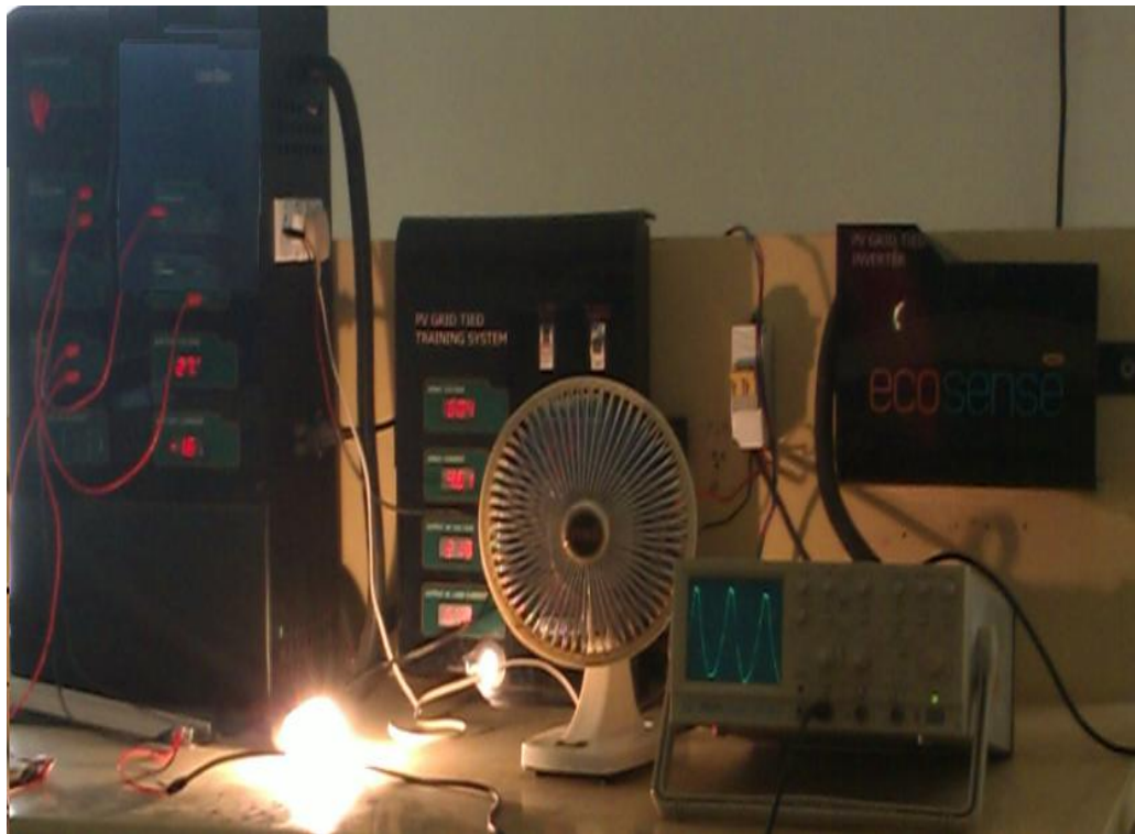
Figure.5 Hardware configuration of PV grid tied system
