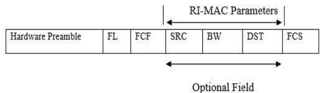
Fig.2 RI-MAC Beacon Frame Format for IEEE 804.15.4 transceiver. The Standard fields of IEEE 804.15.4 – FL (Frame Length), FCF (Frame Control Field), FCS (Frame Check Sequence)
