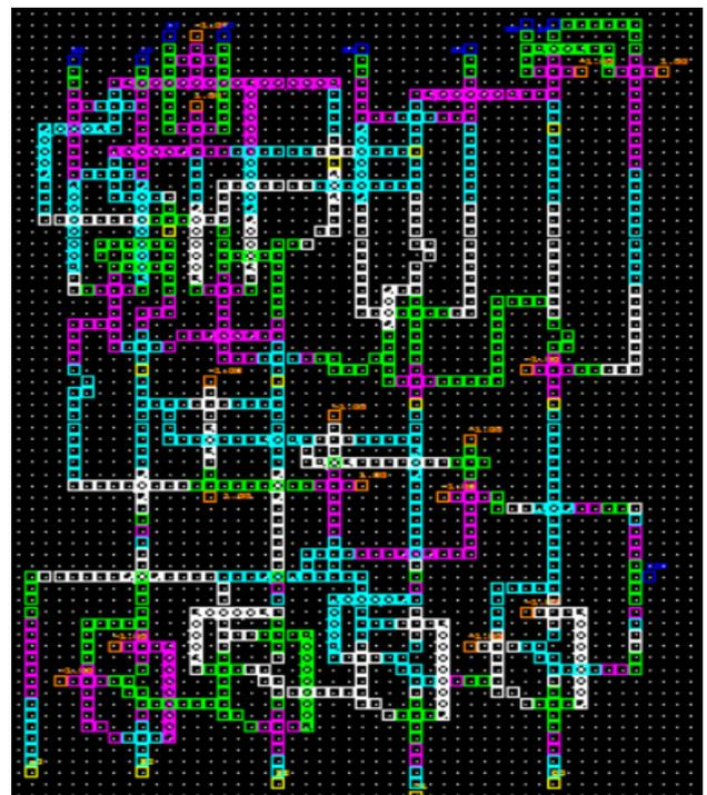
**Fig.2 Layout of BCD Adder**
