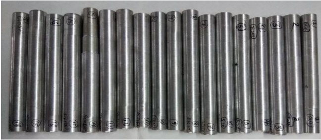
Figure 1. Specimens of Al 7075 reinforced with fly ash and SiC.
