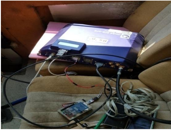
Fig. 13(a) Antenna and NavIC receiver setup for field survey
