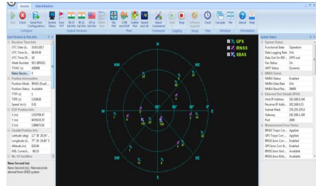
Fig.5. Sky-plot of Various location of NavIC/GPS/SBAS satellites by NavIC receiver
