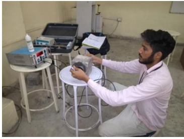
Figure 7 Ultra pulse velocity test
