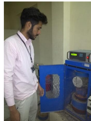
Figure 3 split tensile strength test
