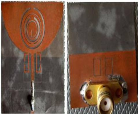
Fig. 2. User model of hexa notched antenna.
