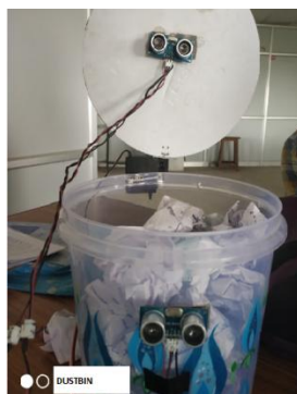
Fig. 9 Fixing of the Ultrasonic Sensor
