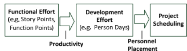
Fig. 1 Size relation to effort and scheduling (Raith, F., Richter, I., Lindermeier, R., &Klinker, G., 2013, December)
