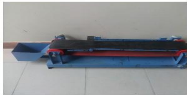
Fig. 3 Belt conveyor setup
