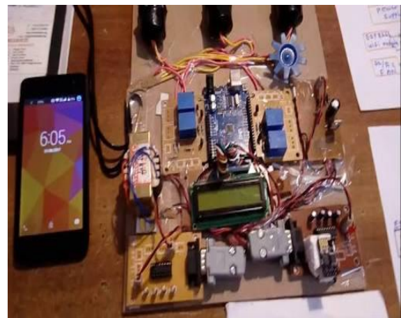
Fig. 7 PIR & IR Sensor based home automation System Saving Energy
